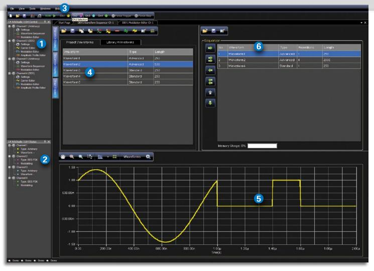
ArbStudio has an intuitive software interface that brings all the important controls to the main screen providing easy access to all channels, output controls, trigger controls and waveform creation screens.
