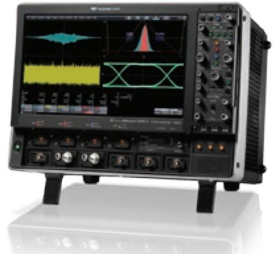
All WaveMaster 8 Zi-A oscilloscopes are implemented with a single hardware platform. To extend bandwidth beyond 20 GHz, Teledyne LeCroy has leveraged DBI technology to minimize initial costs—the module that doubles the bandwidth slides into a separate slot in the WaveMaster 8 Zi-A platform.
