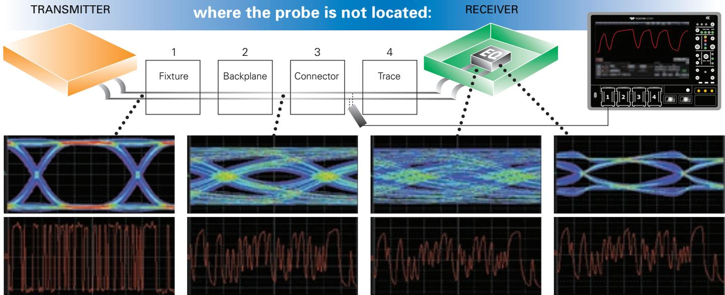
*Virtually probe the signal at the transmitter with the fixture present, and then de-embed its effects from the measurement.*
