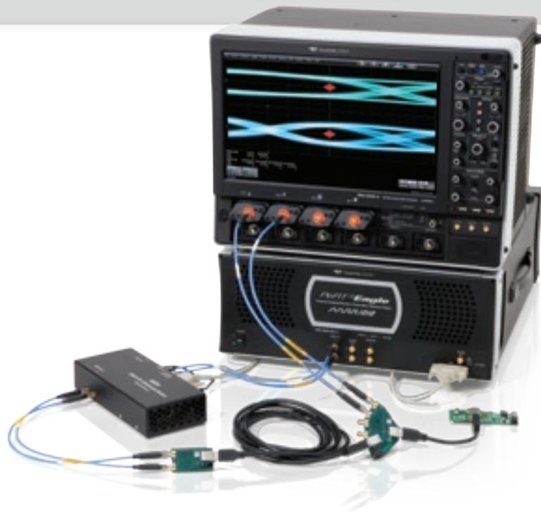
The combination of the SDA 8 Zi-A Serial Data Analyzer, the PeRT<sup>3</sup> and the SPARQ provides the most comprehensive solution for serial data compliance testing. These three pieces of equipment enable a full suite of physical layer compliance testing and debugging ability that will guarantee the best signal integrity for your serial data signals.
