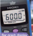
Bar graph refreshes 40 times/second. Acts just like an analog meter to intuitively expose changes in the measured signal.
